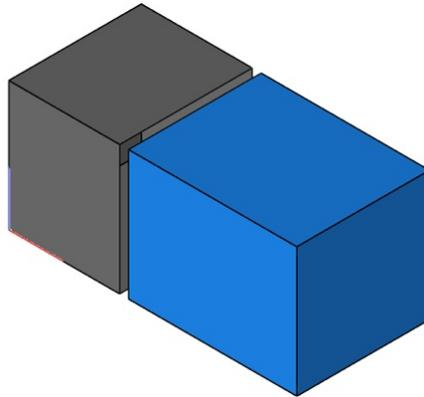
3. Vertices of Mesh 2 that are within the specified distance are moved to Mesh.
