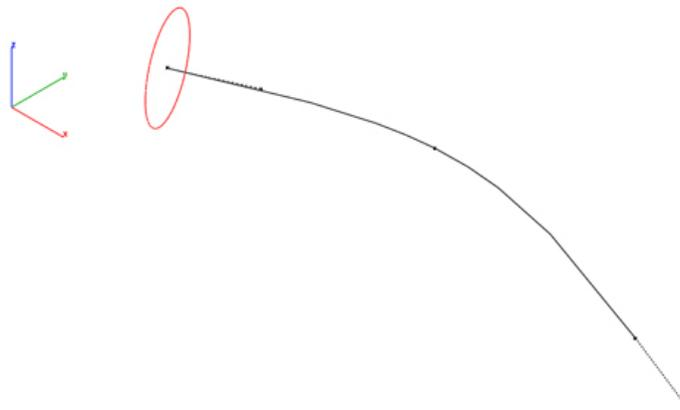
4. As an example use, the circles can be used as a profile of skinned solid.
