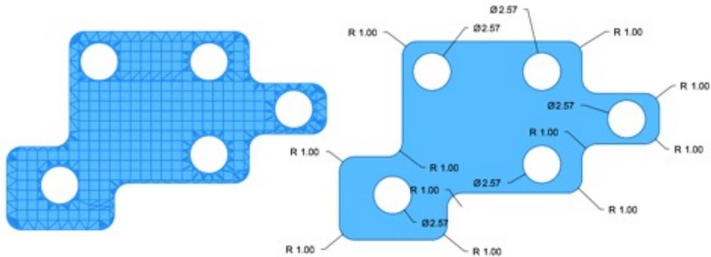
Extrusion : Converts a collection of triangle or quad facets into an extruded solid. Includes conversion of precise cylindrical holes and fillets.
