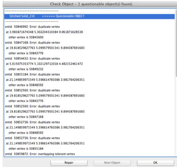
2. Select the Part Repair tool. Part is repaired if possible.
