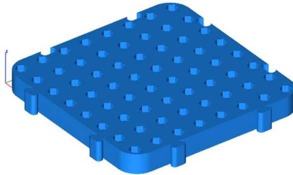
3. The selected mesh is converted into a collection of meshes separated by planar and connected elements. In this example 67 additional mesh objects created.
