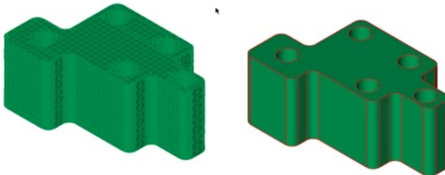
Revolved and Lathed : Converts a collection of triangle or quad facets into a revolved solid. Includes conversion of precise cylindrical holes and fillets. Only full 360-degree lathe and revolved shapes are recognized.
