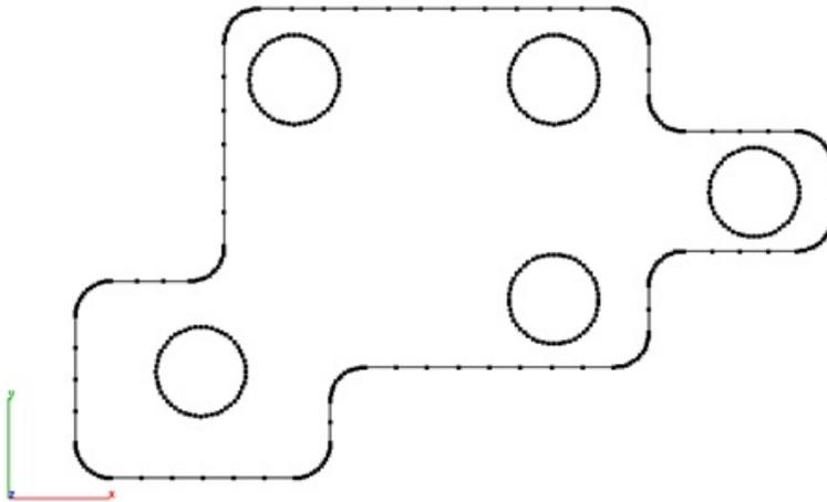
2. Dialog is displayed showing results. In this example, 470 lines are converted into 17 arcs and 13 lines.
