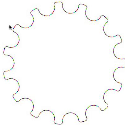
2. Dialog is displayed showing results. In this example, 885 lines are converted into 45 arcs and 31 lines.
