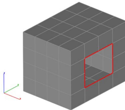
3. Press Undo to remove the red lines located at the mesh free edges.
