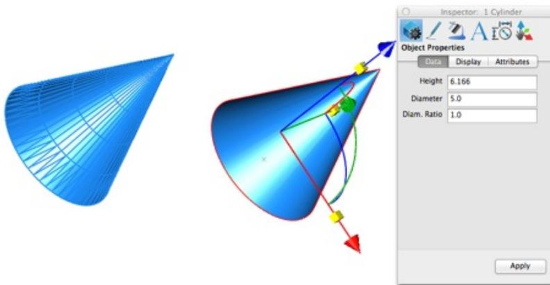
Truncated Cone : Converts a collection of triangle or quad facets into a solid truncated cone defined by height, base & top diameter, and point at base center.
