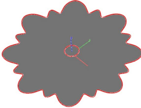
3. Select the Stitch tool to combine the surfaces into a water tight volume suitable for mass property calculations or shelling modeling operations.
