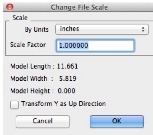
**By Units** Determines the scale factor by converting between units.
