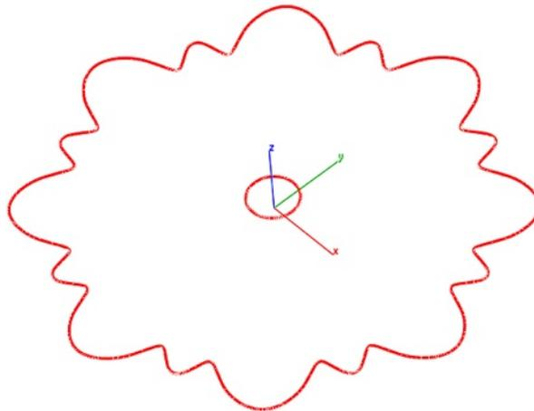
2. Select the Cover tool from the surface palette and select all the curves to create a planar surface.
