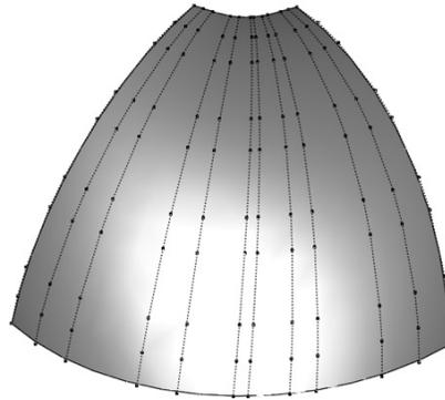
5. Select a reference face or surface. A new surface is created with the specified grid settings.
