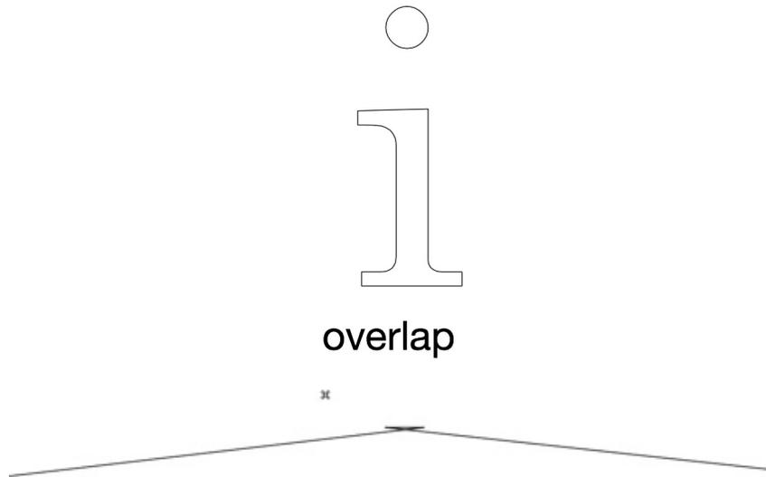
3. Overlap issue detected and repaired. Profile is then suitable for profile based operations such as extrude into a solid.
