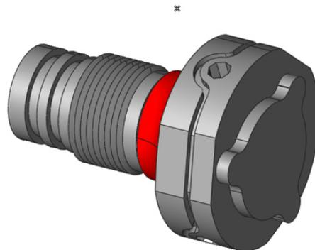
2. Select one face of the protrusion face network. All associated faces will be added to the selection.
