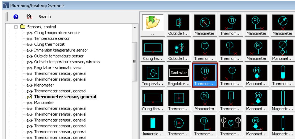
We set the scale as 200 and we insert the *thermometer* symbol into the boiler.
