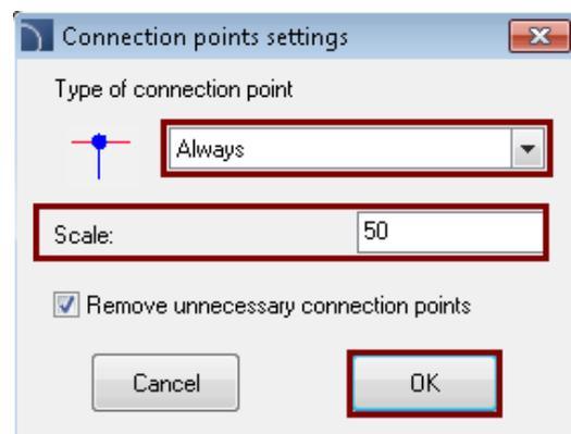
We choose the *type of connection point* as *always*, we set the scale as 50 and next we click *ok* and we draw the line from the *heater* to the main *Supply* line.
