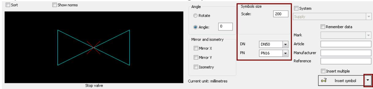
We set the scale into 200, DN into 50 and PN into PN16. We click the arrow that is located next to the *Insert symbol* button and from the drop-down list we choose *Into many pipes* thanks to which we will be able to insert our symbol into many lines. Then, we should specify the edge that crosses the lines. That's why we click in the P1 point first and next into P2 point. Symbols will then be inserted in points that are being crossed between our selected edge and the lines.
