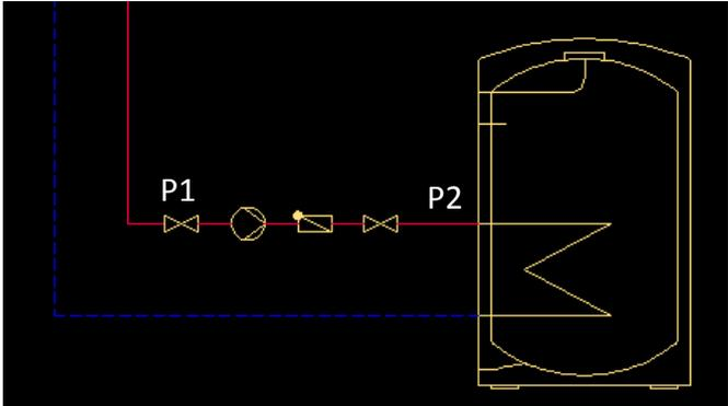
Next thanks to the *Multisymbols* command we will insert the symbols' set as we have put previously. After we have run the command we click the *Most recently selected symbols* thanks to which the last set of symbols will be added into the list (*Stop valve, Stop valve, Pump, Swing check valve*).
