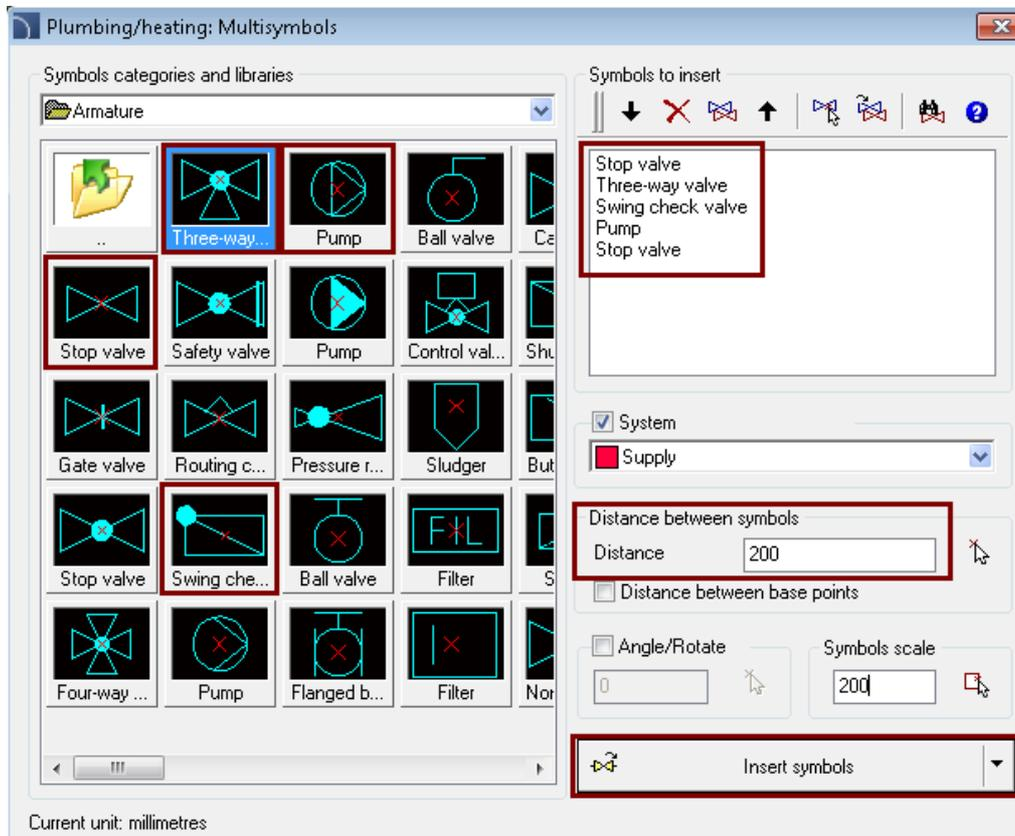
There should be a line between the symbols that's why from the *System* list we will choose *Supply* and we add the distance between the symbols as 200 in the distance box. After we have clicked the *Insert symbols* button we need to show the distributor's stub first (P1) and next we click the (P2) point in such way that the line with symbols will be drawn upwards.
