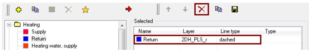
After that we click *OK* and we draw the *Return* line just like in the picture below. In the *Advanced ortho* it is easier to choose to draw three lines simultaneously. In this case we need to click the boiler's exit point and next in the command line choose the option *Three* (you just need to type in the command line *T* and click *Enter*)
