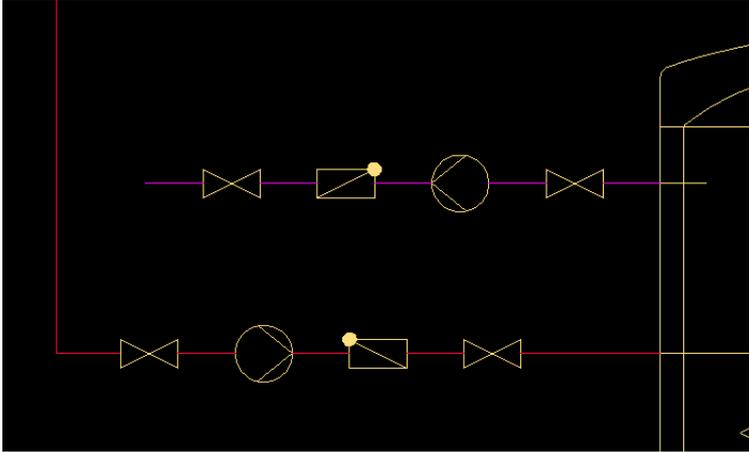
Lets insert one additional *Stop valve* on the *Return line*. We can use the *copy* option that is located in the *Quick edition* command or we can use one of the following commands: *Symbols*, *Multisymbols*, *Insert similar object*.
