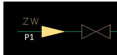
Next we thanks to the *Pipes – scheme* command we draw the *Warm water* line.
