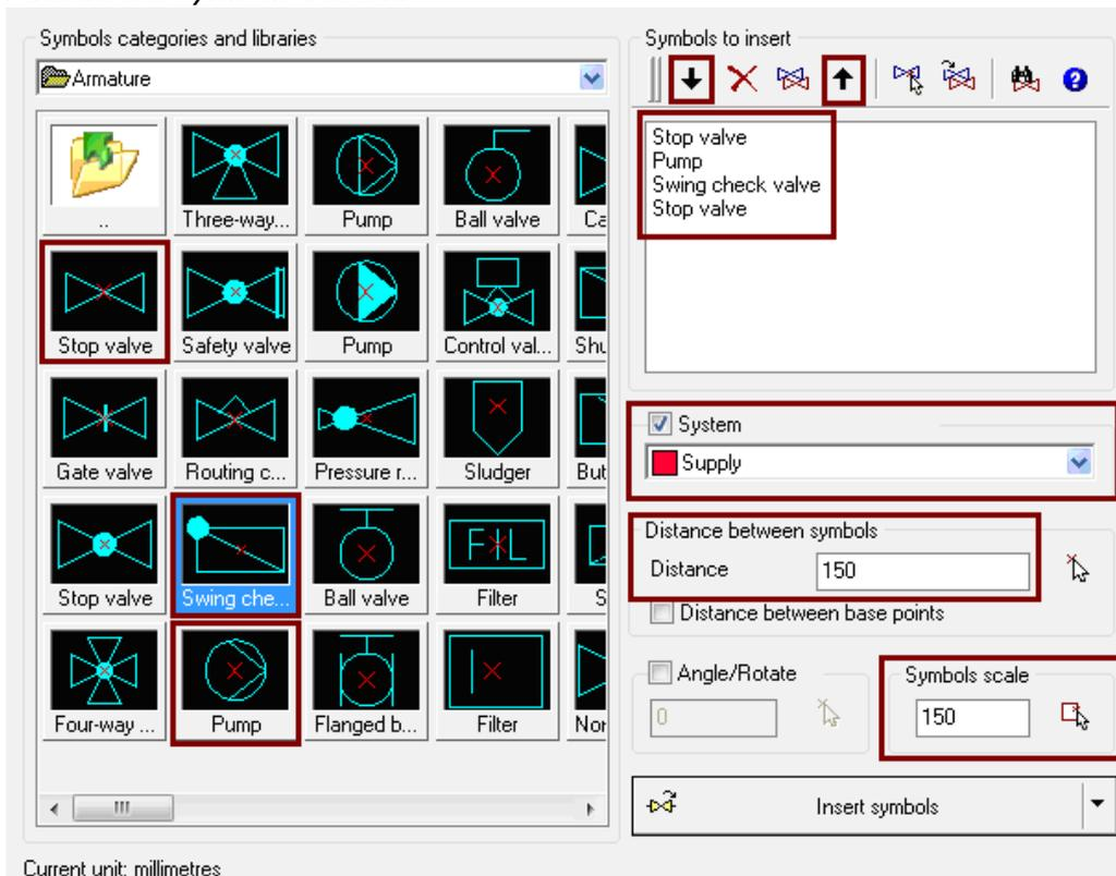
Symbols may be inserted into the already existing line. We indicate the point on the line where the first symbol will appear (P1) and next we choose the direction where we would like to have our multisymbols (P2).
