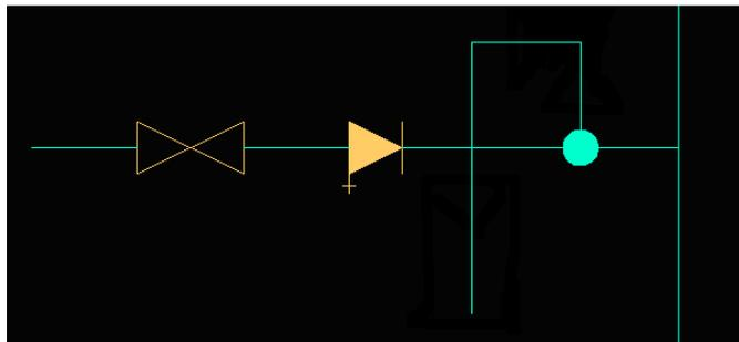
In the next step we will insert a *Overflow valve*. In order to do this we click the Cross symbols button that is located on the HVAC and Piping toolbar.
