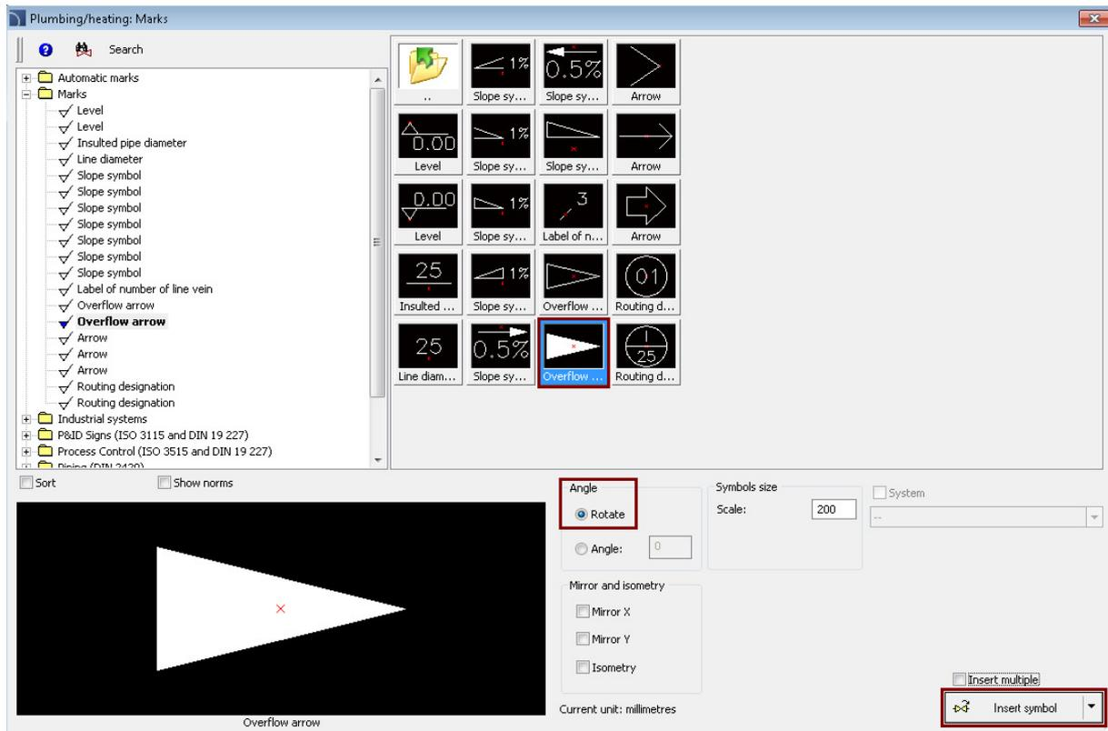
We insert the *Overflow arrow* symbol at the end of the *circulation* line P1. With the selected *Rotation* option we will also need to indicate the P2 point that indicates the edge.
