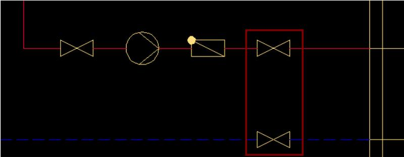
Next we will insert an *Overflow arrow* symbol on the *circulation line*. We click the *Marks* button that is located on the *HVAC and Piping* toolbar.
