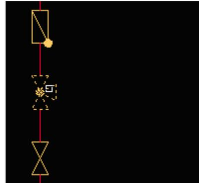
In the dialog window we change the *Three-way valve* into *Three-way valve (multivariant)* – multivariant symbols have got black&white miniatures.
