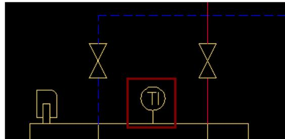
In the same way we will insert a *thermometer* symbol into the *distributor* and the manometer symbol into the *boiler's Supply line*.
