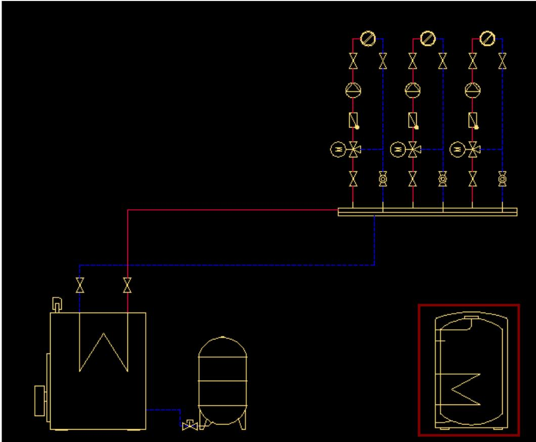
Next we connect the heater with the *Supply* and *Return* lines. We run the *Pipes – scheme*
