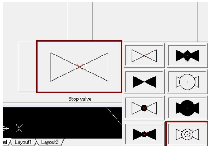
After we have chosen the right valve we can insert it into the *Return line* by clicking the *Insert symbol* button. We can use the *Into extension* option that will allow us to precisely insert the symbol at the same level as the *Stop valve* symbol.
