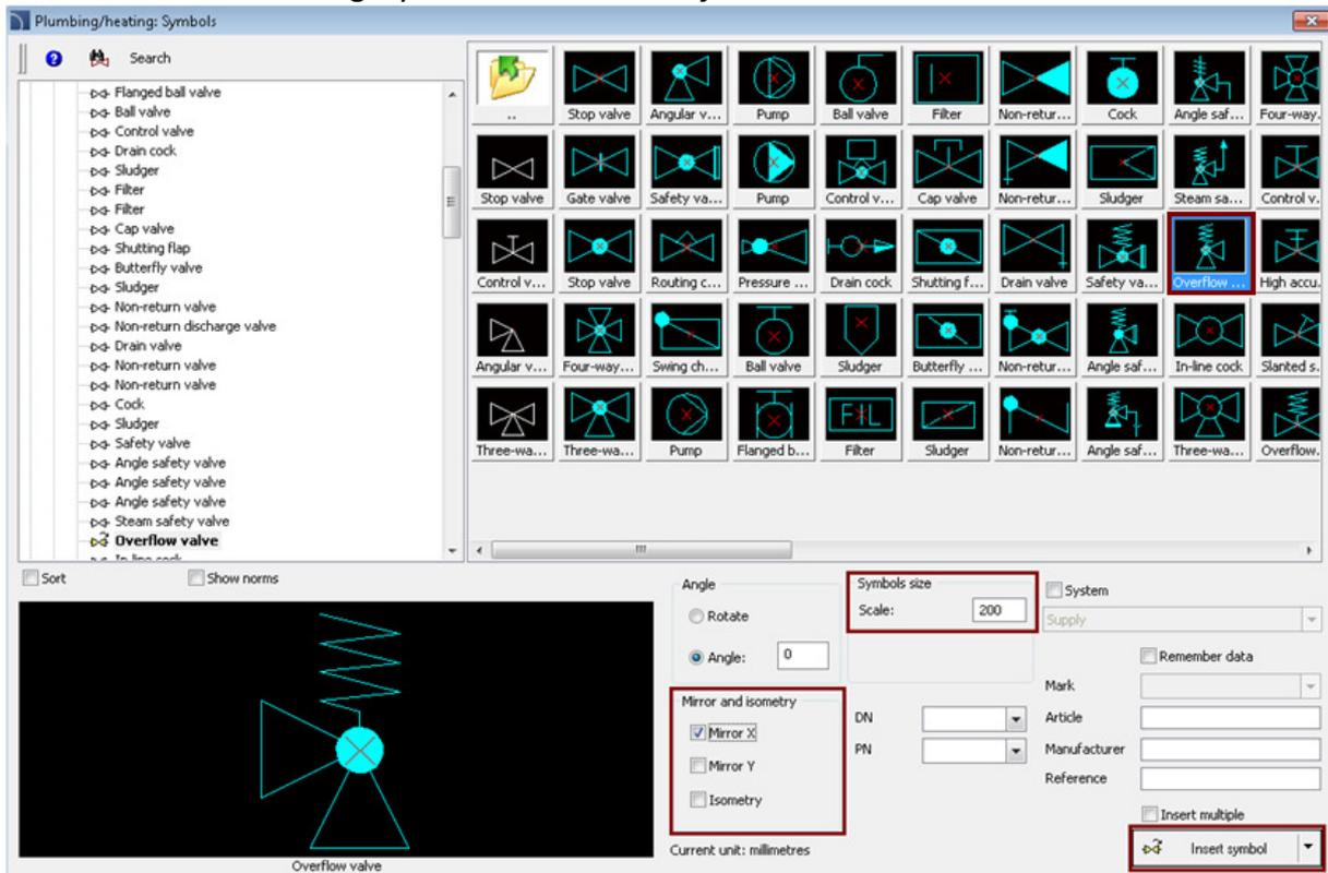
We set the symbol's scale into 200, we check the option *Mirror X* and after that we click the *Insert symbol* button and we insert the *Overflow valve* in the place that is shown on the right picture.
