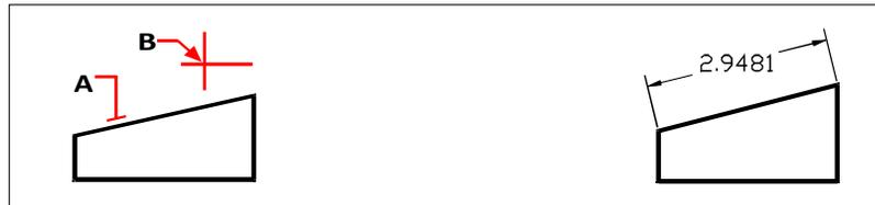
To insert an aligned dimension by selecting the entity, select the entity (A) to dimension, and then select the dimension line location (B).
