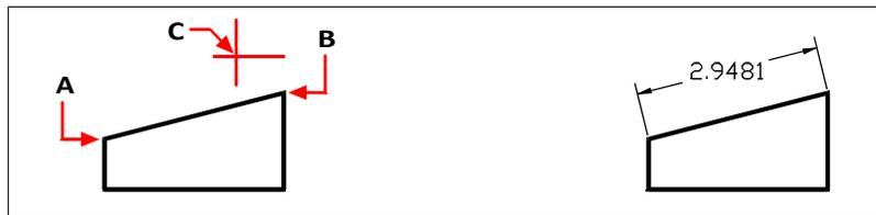
To insert an aligned dimension by selecting the extension line origins, select the first extension origin (A), select the second extension origin (B), and then specify the dimension line location (C).
