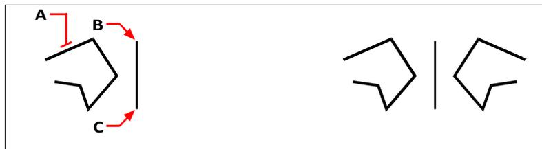
To mirror an entity, select it (A), and then specify the first point (B) and second point (C) of the mirror line.
