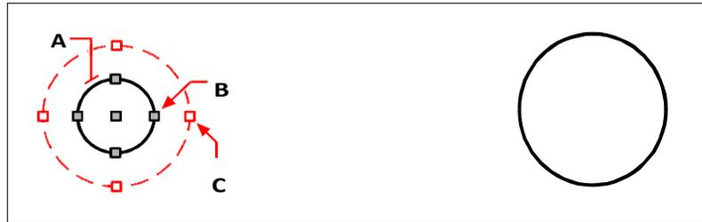
To scale using grips, select the entity (A), click a grip (B), and scale the entity by dragging the grip to its new location (C).
