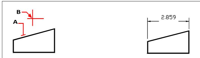
To insert a linear dimension by selecting the entity, select the entity (A) to dimension, and then specify the dimension line location (B).
