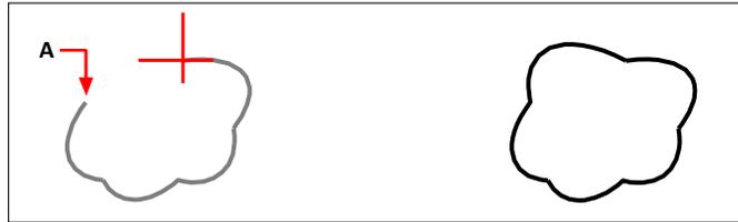
Select start point (A), then move the mouse around the desired area and back towards the start point (A).
