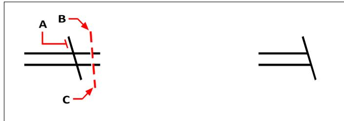
Select the boundary edge (A), and then specify the first point (B) and second point (C) of the fence.
