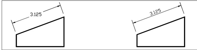
Text between extension lines aligned horizontally.
