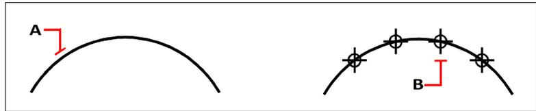
When you select the entity by pointing, divisions are marked beginning from the end closest to the point at which you select the entity (A). Blocks or point entities (B) are placed along the entity to mark it in equal intervals.
