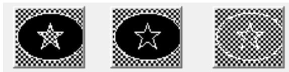
Nested islands (A), with outer island (B), and with ignore islands (C).
