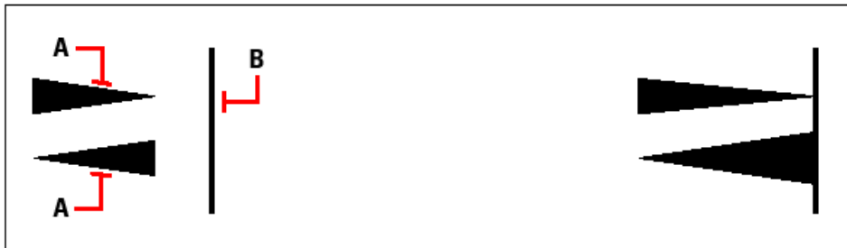
A tapered polyline (A) continues to taper until it intersects the boundary edge (B).
