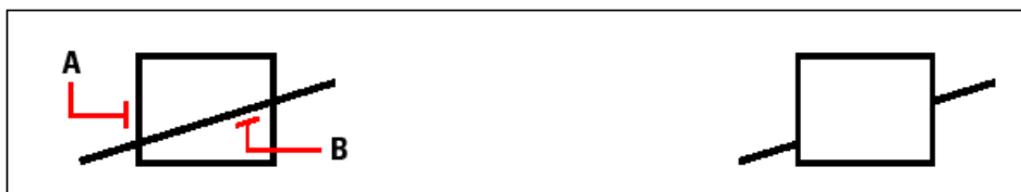
To trim entities, select the cutting edge (A), and then select the entities to trim (B).
